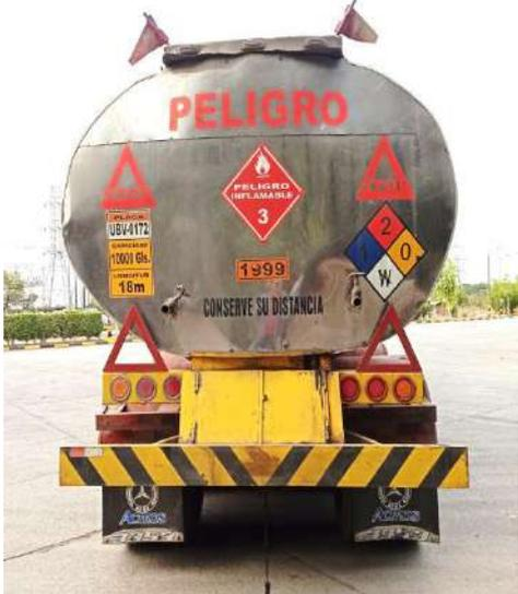
A rear-facing photograph of the tanker truck. The tank is silver and has 'PELIGRO' written in red. There are several hazard labels: a red diamond with a flame (3), a blue and yellow diamond with '2' and '0', and a white diamond with 'W'. The text 'PELIGRO INF. LAMABLE' is visible. The truck has a yellow and black striped bumper and a license plate that reads 'UBV-172'. The year '1999' is also visible on the tank. |
